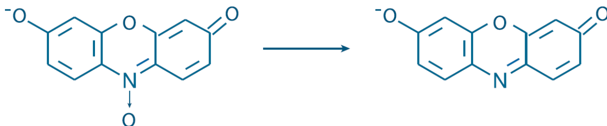
Figure 1A. ViaBlue™ serves as a reliable cell viability and proliferation indicator by measuring the reduction of resazurin, a non-fluorescent dye, to resorufin, a highly red-fluorescent compound, through the metabolic activity of living cells, with the resulting fluorescence intensity being directly proportional to the number of viable cells.
